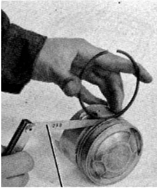
Fig. 3.24 Piston ring side clearance in the piston
