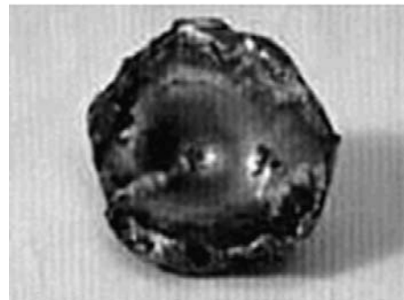
Valve head broken off
