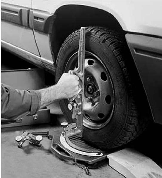
Fig. 22.41 Camber gauge in position (Sealey garage equipment)
