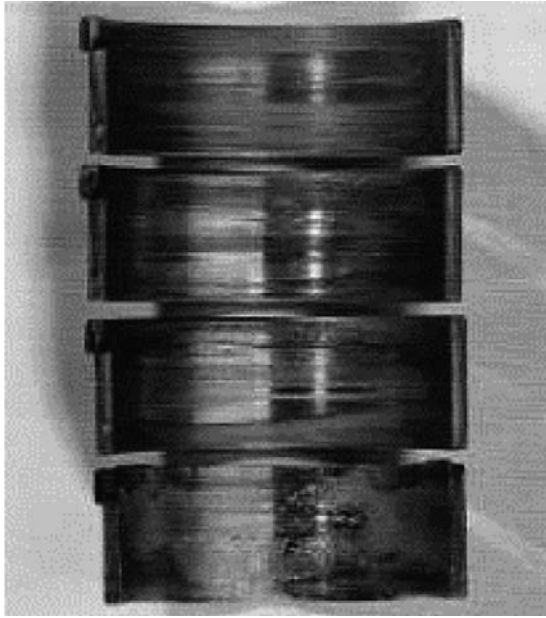
Fig. 17.7 Big-end bearing failures
