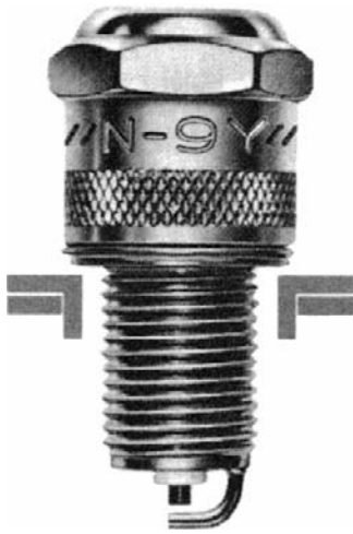
Fig. 27.50 A gasket-type plug seat
