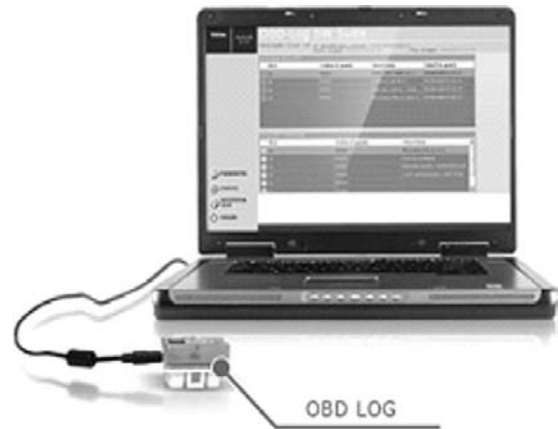
Fig. 29.16 The Texa OBD data logger
